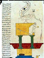
Figure 6: Drawing of the water-lifting machine described by al-Jaziri in his Book of the Knowledge of Ingenious Mechanical Devices. The drawing is a detailed illustration of a mechanical device, likely a water-lifting machine, with a vertical shaft and a bucket-like structure. It is labeled with Arabic text.
